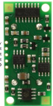
+5v Echo output Trigger input Do not connect GND
